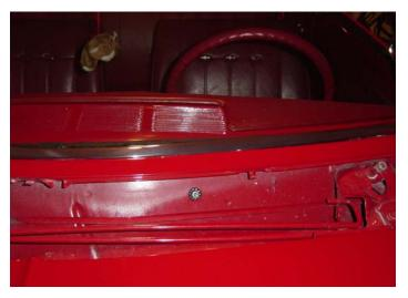
If your car doesn't have a dimple, I'd recommend you use your brace itself to locate where the hole in the plenum-chamber wall should be by attaching the dash end of your brace to the reinforcement, with the end of the brace aligned parallel to the car's centerline, and making your own dimple.
