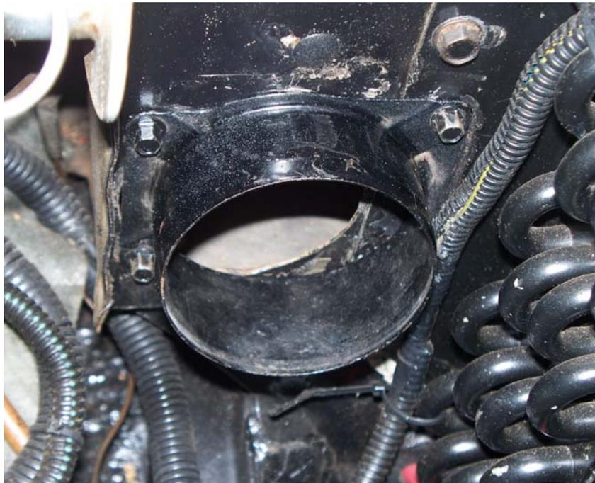
so that he could attach a(n extra) hose connector from the cool-air intake of the heater found at the front of the engine's top shroud. This connector, which attaches very simply with three screws, calls for 3-inch air hose, which Wade attached with the usual clamp and routed to the air cleaner.
