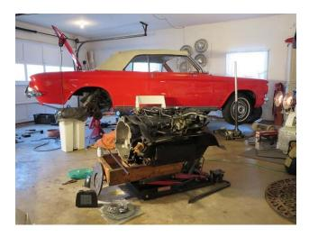
With the snout fixed and a new input shaft procured, Bob Marshall installed the new clutch components while the rest of us stood around and made snarky comments. (In all fairness, Ron Tumolo did an outstanding job keeping the engine from turning as Bob tightened the various components.) The highlight (for me, anyway), was refilling the transaxle by removing the top cover. At first blush this has to be the
