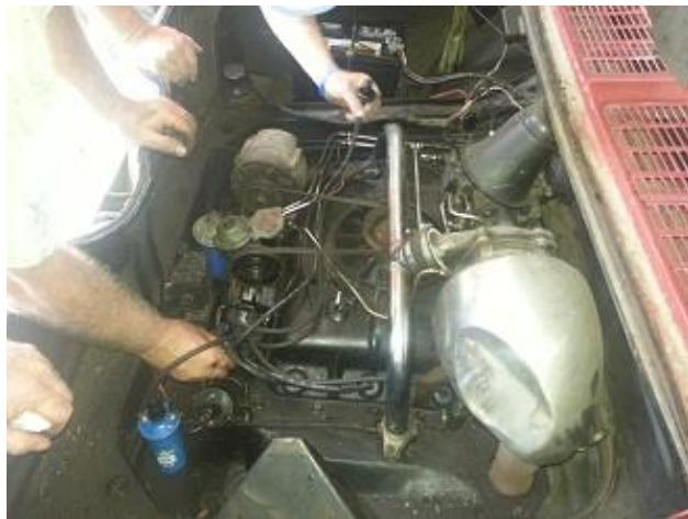
Suzi now has a decision to make regarding how far she wants to go in resurrecting her Corvair. Like any old car that's been sitting for more than a decade, the gas tank will have to be drained and de-varnished; brakes, fuel lines, and tires will have to be replaced; and the carb will have to be rebuilt. In any event, it would be thrilling to see this rare Corvair motivating under its own power once again!
