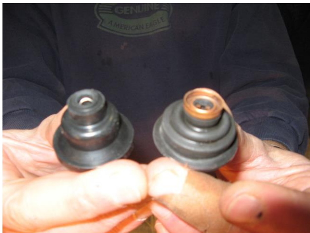
The washer diaphragm thingy – new and old.
