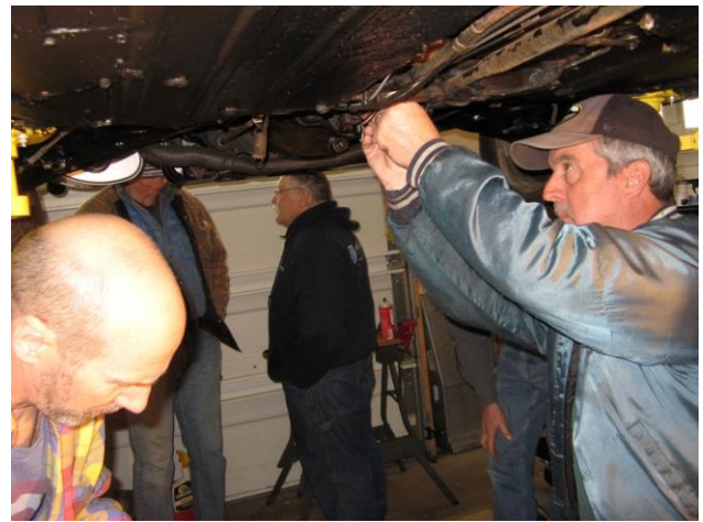
Running the e brake cable.
