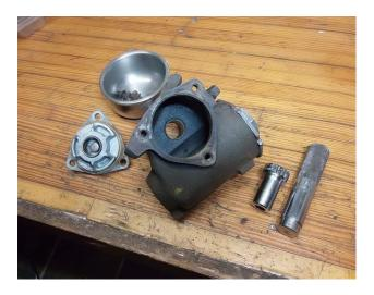
The upper driver is the installer, lower is the remover. The remover shoulder bears against the bushing and you drive it though the hole, the installer has the shoulder, so you don't go too far. If you look carefully at the remover in the photos you can see how it's been mushroomed.
