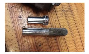
The remover post filing. Note the finish is filed off and you can see the end was deformed enough that it's no longer square to the shaft.
