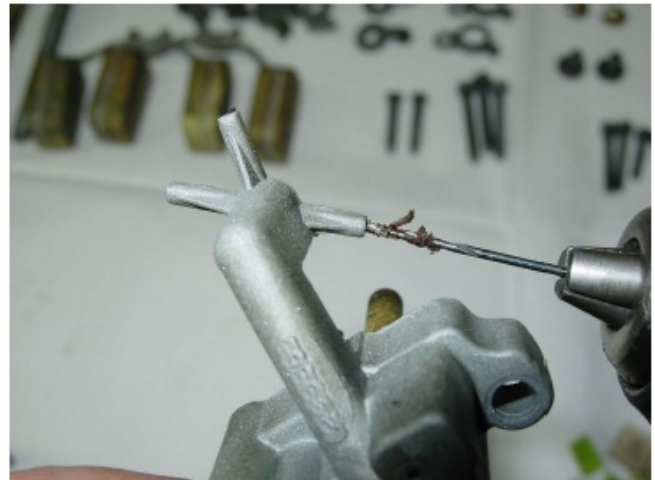
Totally plugged discharge nozzles being cleaned with a #56 drill bit.
