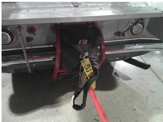
Note push bar below the chute, trip hazard
