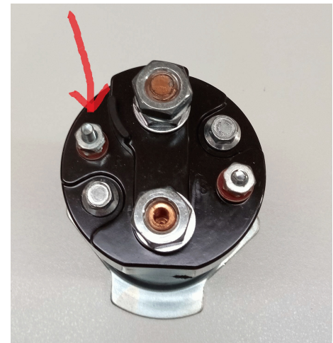
The terminal on the left is the resistor by-pass and should show battery voltage anytime the key is turned to start.
