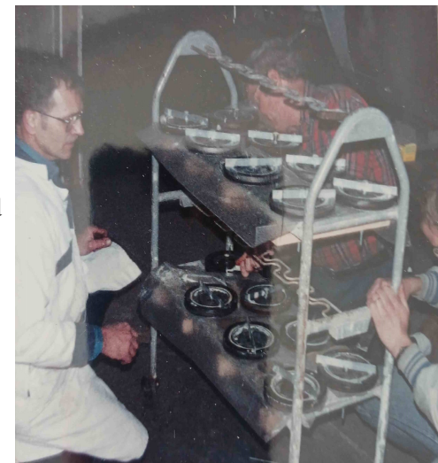
Norman Laubach and Gerry Burnett during harmonic balancer rebuilding session
