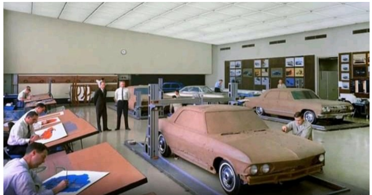
Clay model to study the 1965 Corvair. (photo courtesy of General Motors)
