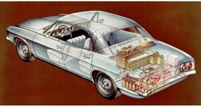
Easily the most distinctive feature of the Electrovairs was their batteries. Both used silver-zinc cells, a type more often found in aerospace and military applications. Electrovair II used 286 silver-zinc cells wired in series and arranged in 13 trays with 22 cells per tray. Seven battery trays were mounted in the front luggage compartment, while the other six trays were installed in the engine compartment out back
