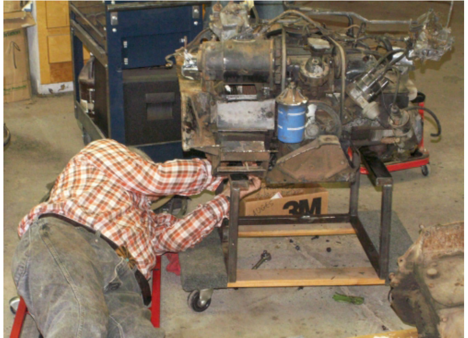
ABOVE: Lloyd Folger works are adding thread inserts into stripped pan bolt holes. He found several bunged up threads when he resealed the oil pan. Strecker photo
