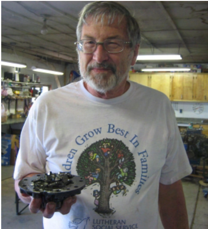
ABOVE: Larry Lee hold the remains of his Spider gears. Dan Hagenbuch photo
