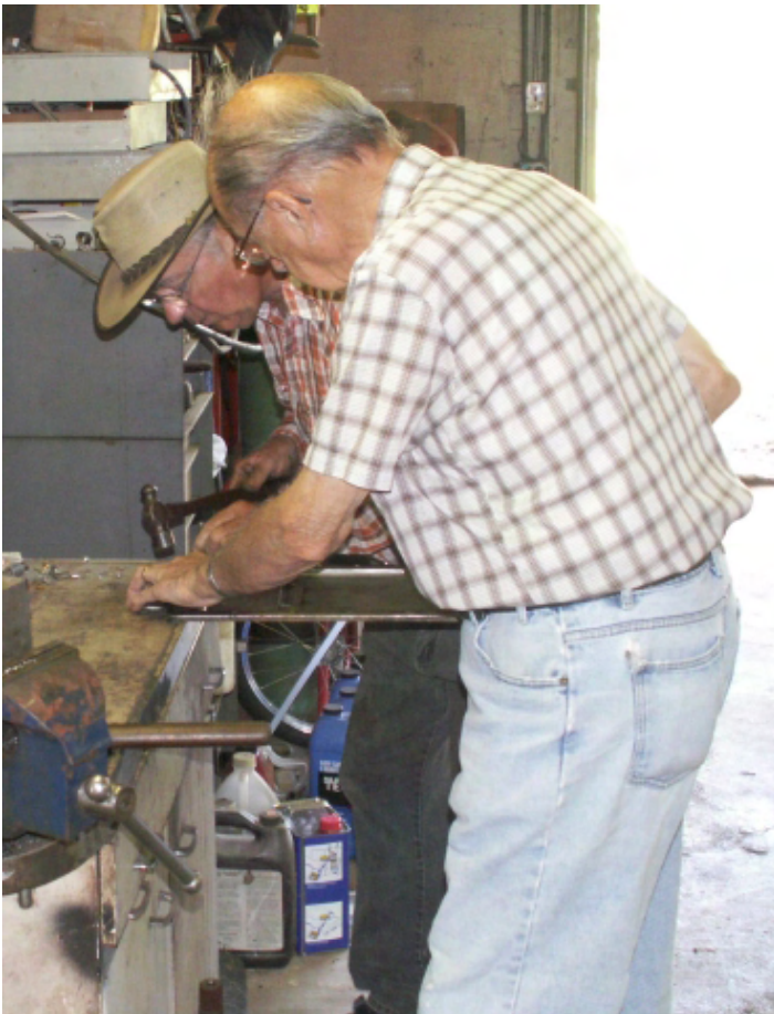
ABOVE: Mel Horstman helps Lloyd Folger flatten the sealing flange of his oil pan. Lloyd was replacing the pan, bellhousing, flywheel and clutch on an engine he was mating with a transaxle. Strecker
