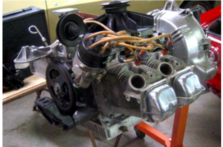
ABOVE: The experimental engine looks much like a production Corvair engine, but the individual valve covers and generous intake ports indicate some of the differences lurking deeper within.
