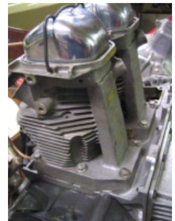
Cylinders and heads were cast as one unit.
