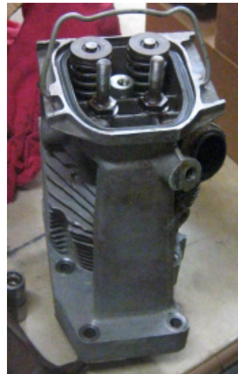
ABOVE: The experimental engine looks much like a production Corvair engine, but the individual valve covers and generous intake ports indicate some of the differences lurking deeper within.
