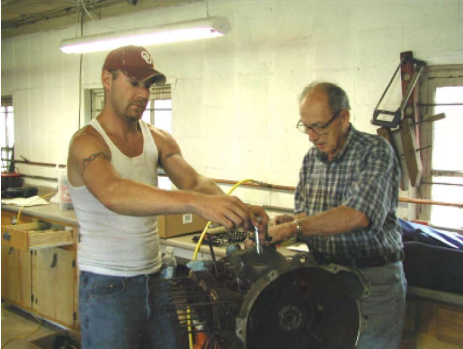
2004 Bernie Streker's son, Justin, helps Mel Horstman tear down a Corvair engine. Mel plans to combine the best parts of this engine with parts from an engine he tore down at Cold Tuna to make one good engine.
