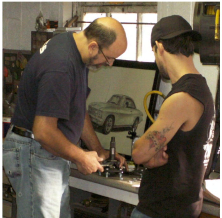
At last year's Tuna, Tom Horstman and son Tommy from Dallas measure the end play on a pair of Late Model rear wheel bearing assemblies they rebuilt for Tom's 67 convertible. Strecker photo.
