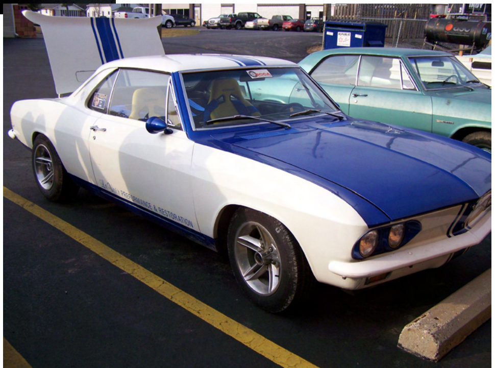
LEFT: Yet another Stinger owned by Warren Le Veque (Michael’s father). This Yenko is an all-out race car, extensively lightened and powered by a highly modified Corvair Turbocharged engine.
