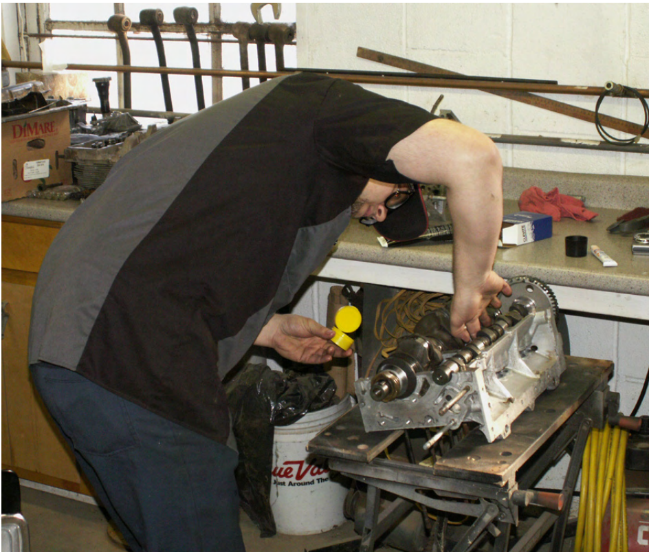
LEFT: Starting the day with bare block halves and boxes of new and refurbished parts, Ryan Verthein started assembly of his 140 hp Corvair engine. Ned Madsen told Ryan that the block would be together before Ryan's first donut. Ned was right
