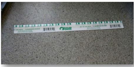
Here's how it works. Cut small pieces of the plastigauge and place it on the surface of the journals you are going to check. To do the main bearings for example, install your bearings in the block halves. Place the crankshaft in one half of the block. Be careful not to spin it around too much as there is no lube on the bearings at this point.
