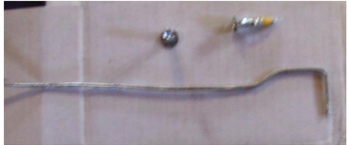
Here are the parts required for the conversion in addition to the choke coil: a 1/16" stiff rod bent to clear, a self tapping screw and a 1/4 inch "molly" style wall anchor.
