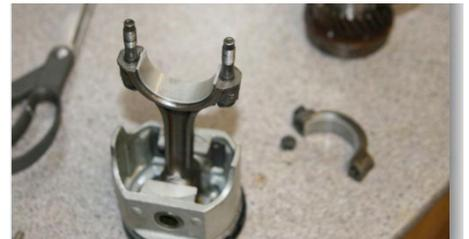
Connecting rod and piston with new bearing installed.
