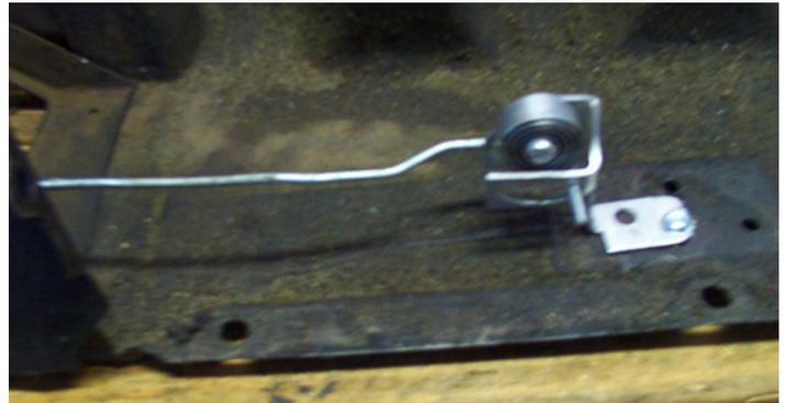
After straightening out the 90 degree bend next to the coils cage, position the foot securing with a self drill/tapping screw. Expand the anchor in the pivot in the door, remove the screw and attach the rod with a 90 degree bend.
