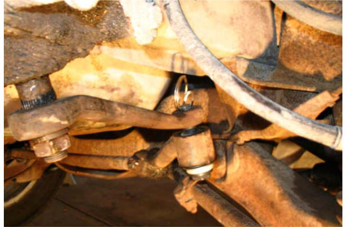
hold it there. Key ring goes through the cotter key hole. Did have tool box, and pliers bent the key ring so it won't just fall out.
