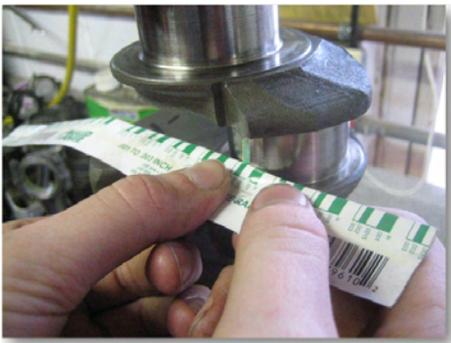
Measure the compressed plastigauge with the packaging and compare the measurement with the spec in the shop manual. In this case the spec was .0012 to .0027. This journal is in spec. Plastigauge is quite a bit of extra work so why do it at all? After all the crank was turned to a spec and bearings were purchased to match that spec. What could go wrong?
