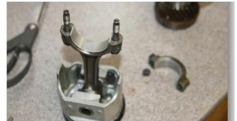
Connecting rod and piston with new bearing installed.
