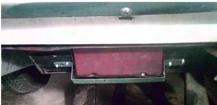
Matt also devised a method to work both thermostat flaps with one working thermostat. Remove the inoperative thermostat and rod, then attach both doors together with a 1" x 24" strap bent to allow the doors to open without hitting the engine.
