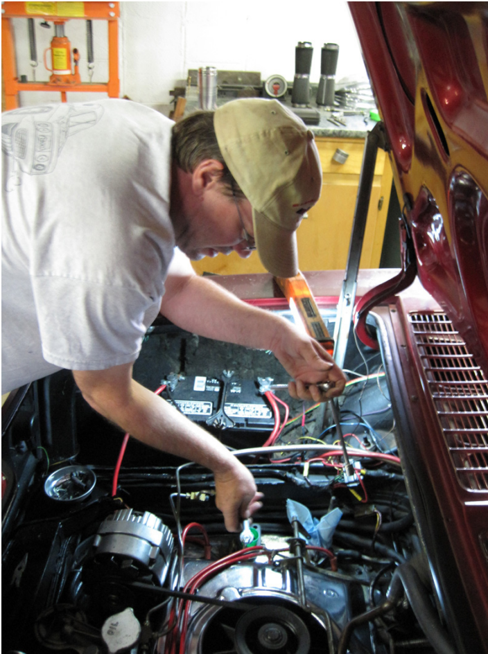
ABOVE: Ned dove in on Chris Teers Convertible. Not only did the carbs need rebuilt, they needed correct studs and choke mechanism installed. The major problem was that the seat for the needle in thee primary carb backed out limiting fuel flow.
