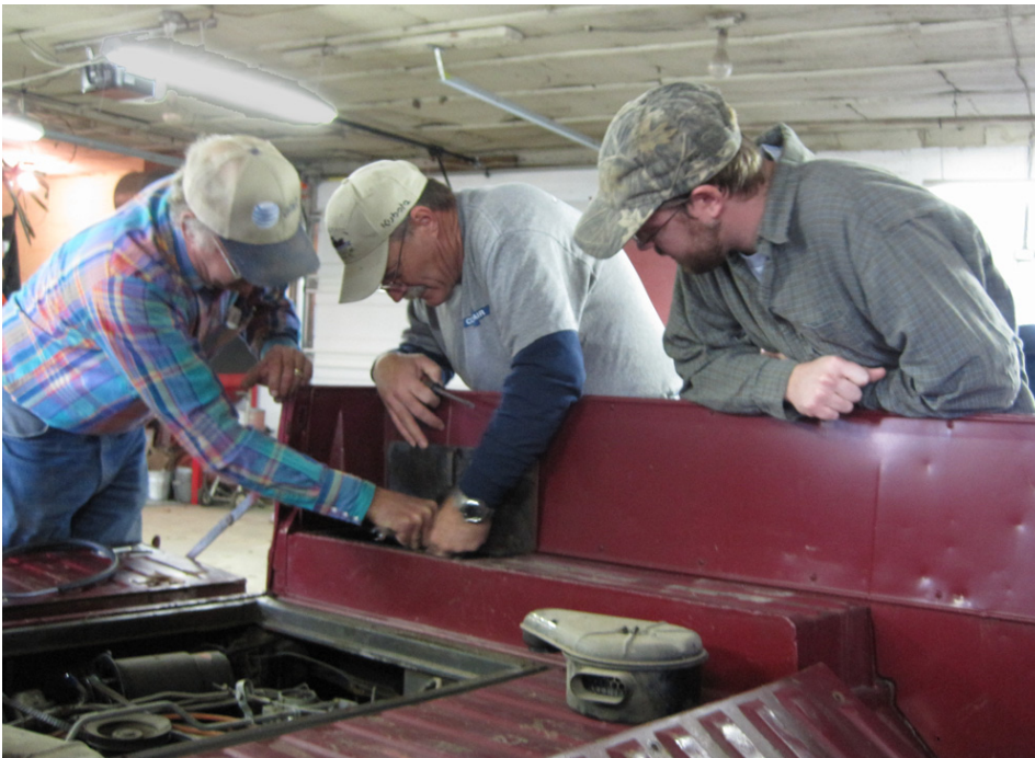
ABOVE: Ned dove in on Chris Teers Convertible. Not only did the carbs need rebuilt, they needed correct studs and choke mechanism installed. The major problem was that the seat for the needle in thee primary carb backed out limiting fuel flow.
