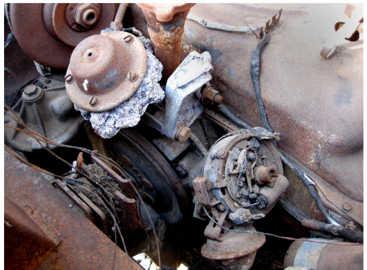
Most rubber, wiring and pot metal parts suffered damage during the engine fire caused by a broken plastic fuel filter in the engine compartment.
