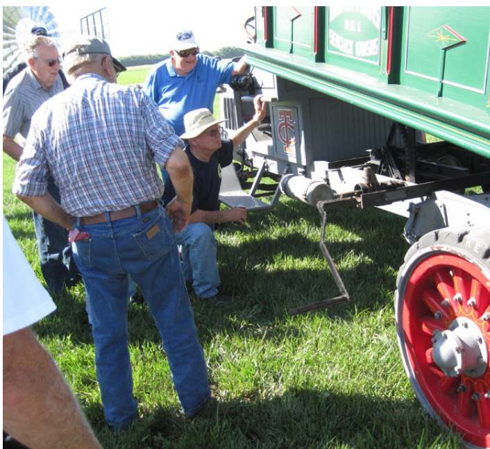
ABOVE: Joe shows off the mechanical dump mechanism of his solid tired farm truck. Doesn't seem like Joe collects anything small.
