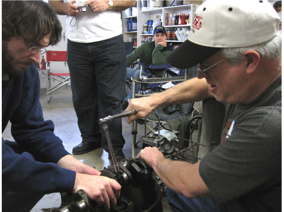
Scott Allison (right) torques down a rod nut while Travis Bolton (left) stabilizes the crank assembly while using Plastigauge to determine the rod bearing clearance. Scott was demonstrating the proper methods to use Plastiguage for the Kansas City Tech session.
