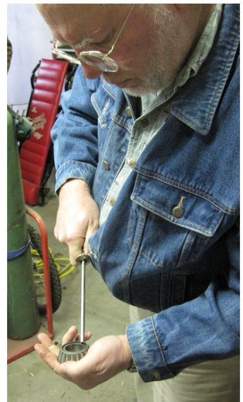
BELOW Wichita Gary Moore blows out some bearings for a LM rear axle rebuild.
