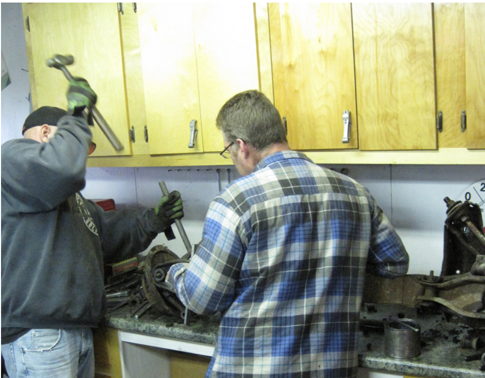
Hammer Time. LP and Alan knock loose the LM front end's ball joints
