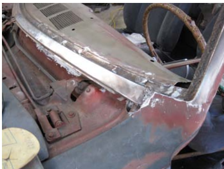
After countless trials, cutting and fitting, the Corsa's new dash and lower panel are welded and ready for filler.
