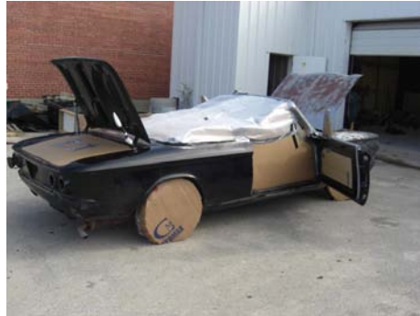
Bryan Easterwood decided to get his '64 convertible media blasted down to bare metal. Since the media gets everywhere Bryan spent the morning, double and triple masking his car for the blaster
