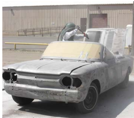
Blasting almost finished. Bryan replaced the rusted front panel and now is ready for minor bodywork and a nice paint job.
