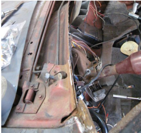
By the time all the rust was cut out, there wasn't much left of the dash and lower windshield
