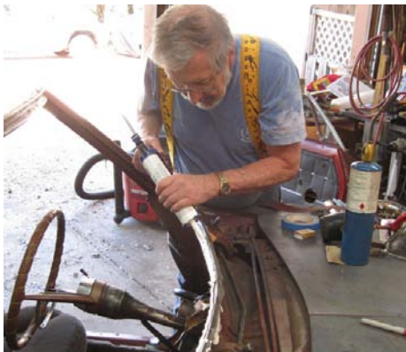
Larry applies a bead of seam-sealer after the brace has been welded. Ready for the cover.
