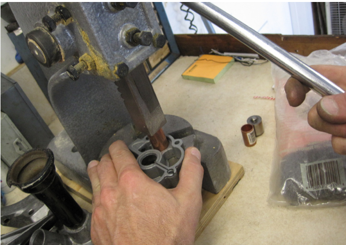
A small press and a copper tubing driver is one way to fully seat the valves.
