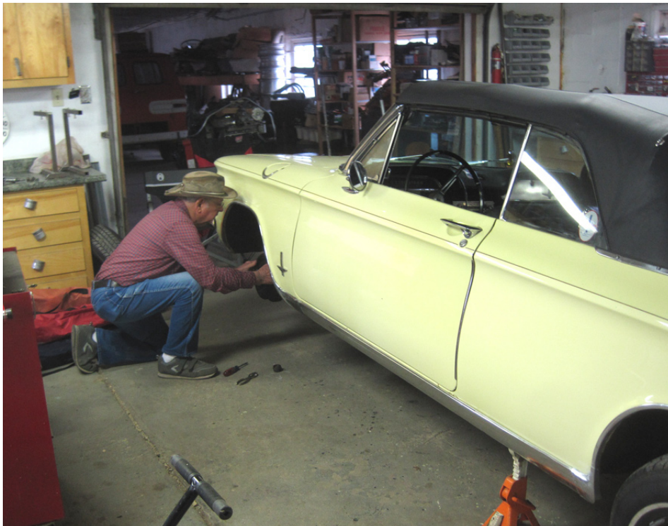
First project of the day was Lloyd Folger's '64 Corvair convertible. What started out as a brake hose replacement wound up being a brake cylinder rebuild when some stuck wheel cylinder pistons were found. Several people helped Lloyd during the day.
