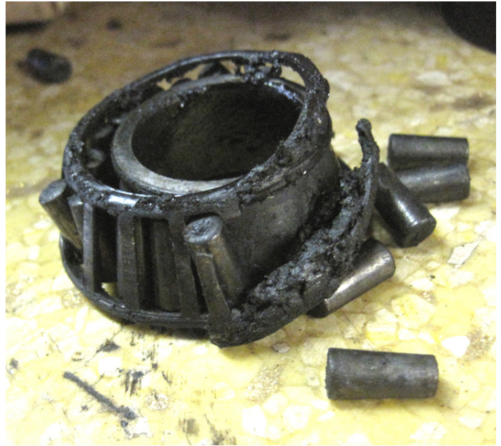
This rear wheel bearing came out of Alex Moat's '68 with a little over 50k miles. Lube had dried out.
