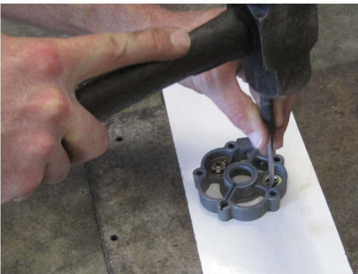
To stake the valves, use a solid base, a small punch and a large hammer. Staking holds the valves in.
