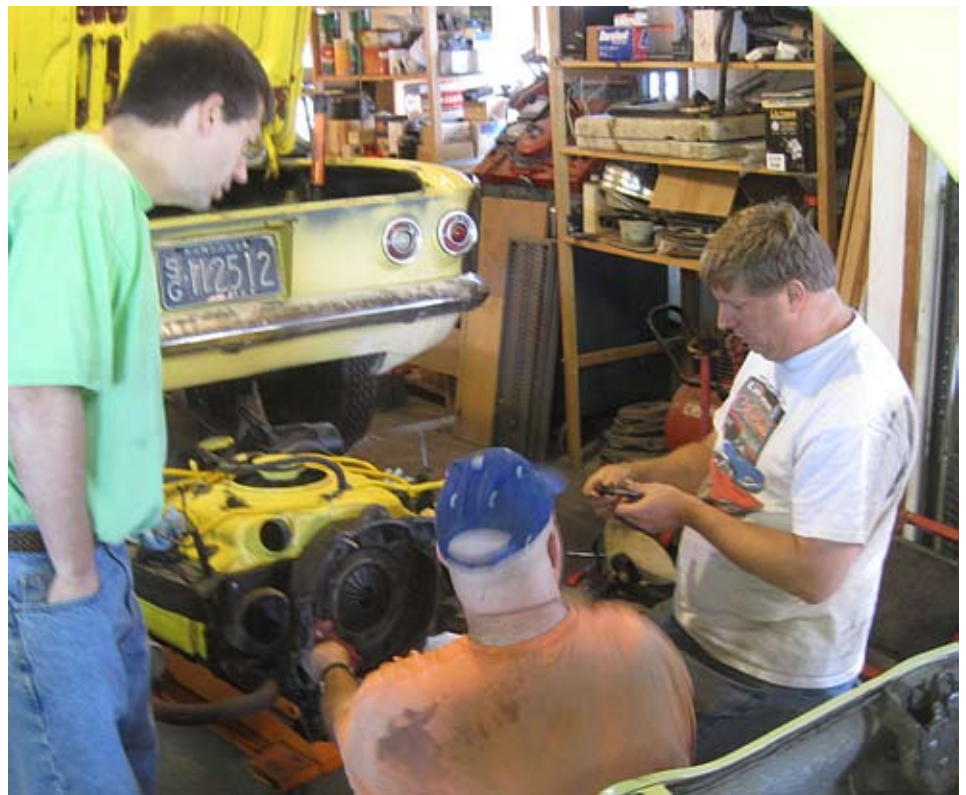
Bryan Easterwood looks on as Jared Strecker and Greg Renfro prepare to pull the clutch and flywheel, then reseal the front of his engine. To see what they found check out the story on page 6.
