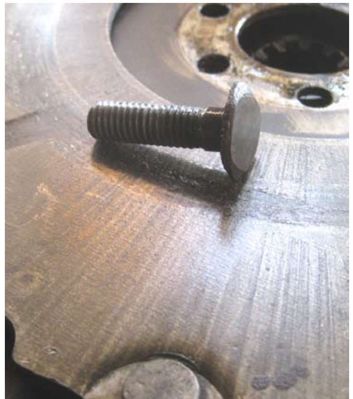
This bell housing bolt had the head reshaped as it loosened up and rubbed on the flywheel
