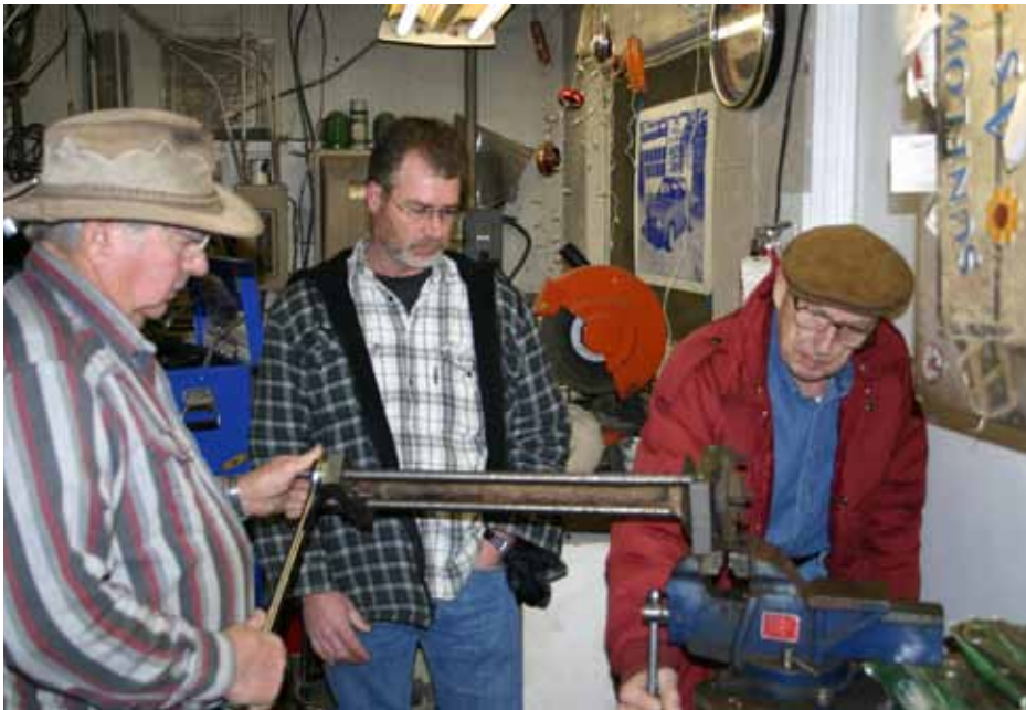
Cold Tuna 2007. Lloyd Folger (left) Alan Ballard and Mel Horstman team up to pull the rear axle bearing off an EM axle. The special tool was purchased by the Club and is available for use at the Kalp Shop. Terry reports the puller is working great as he recently removed the bad bearings from two axles the Chris Teer recently brought up to the shop.
