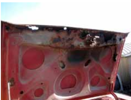
BELOW: Check out the rust on this LM engine cover on a parts car at Wes' shop. Maybe the rust in Wichita is not so bad.
