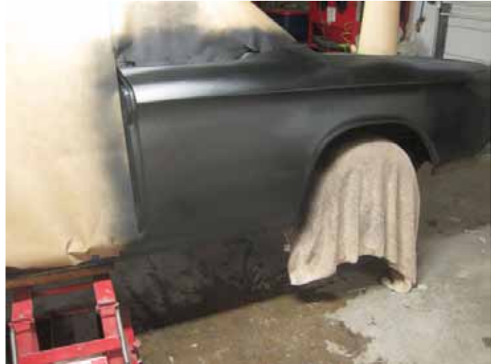
Several skim coats of body filler and the quarter was ready for some John Deer Blitz Black paint.
