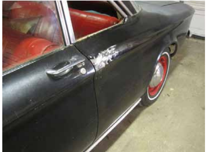
After a session with the Port-a-power the major part of the dent is gone and only a few wrinkles are left.
