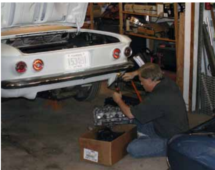
ABOVE: Thanks to Bob Bright everyone had great steak, roasted corn and potatoes. Outstanding job BELOW: Darin LaCrone chips the old exhaust stack gaskets off his recently refurbished heads before installation. Bernie Strecker Photos
