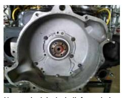
No wonder it leaked oil, four missing bolts. The ones that were there were loose, plus a missing gasket.
