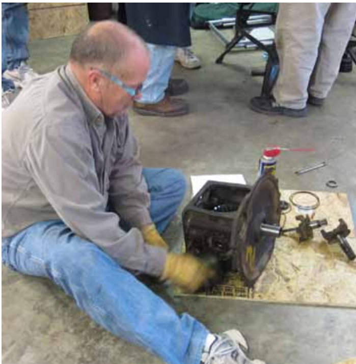
TOP: Kansas City Gary Moore uses an air impact wrench to loosen up the side adjusters on his differential project. LEFT: There were not enough tables for everyone so Gary Jones worked on the floor. After a fresh snout this manual transmission differential was going back together.
