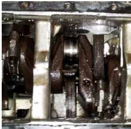
BELOW: On the way home from the Tech session Sam's Corvair developed a bad knock. The source was the missing rod cap.
