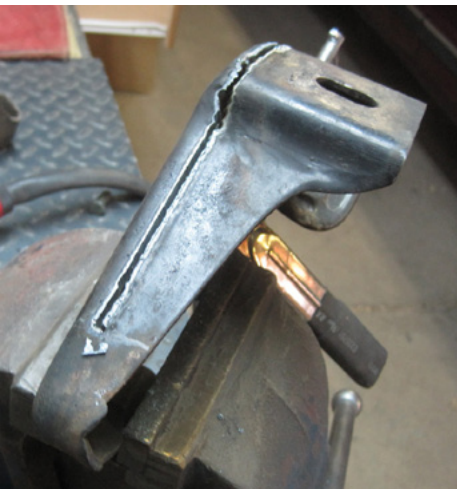
The top part was cut with a plasma cutter. Someone less shaky could have made a straighter cut.
