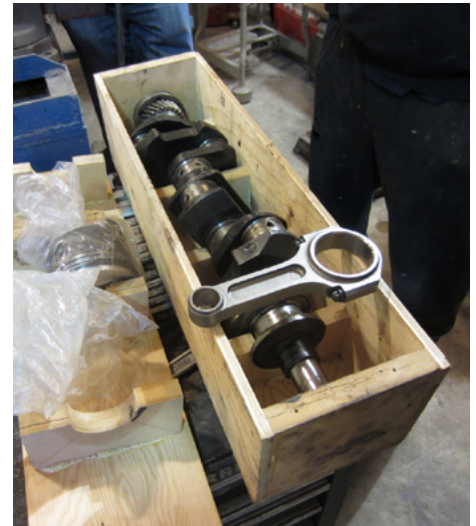
The Box 'O' power belongs to Kevin Willison and contains a 1/2 inch stroked billet Corvair Crankshaft. With oversized VW cylinders it should make a 3.6 liter Corvair engine. Quite an increase over a stock Corvairs 2.7 liter engine
