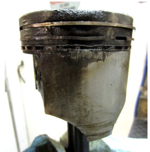
This piston out of Larry Lee's 140 shows damage from the combustion gases eroding one side of the piston. Often caused by detonation.
