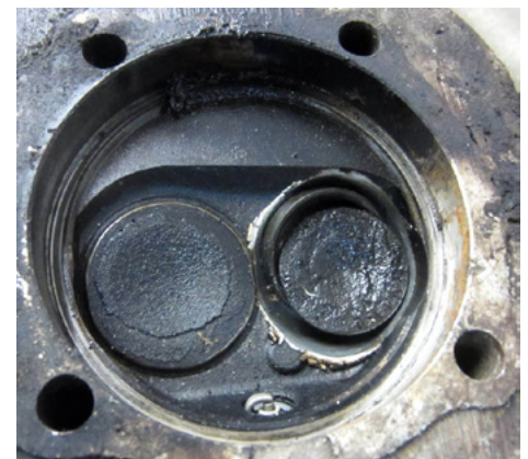
From the other side of the same engine was this dropped exhaust valve seat. Larry was lucky the seat didn't shatter and scatter to other cylinders.
