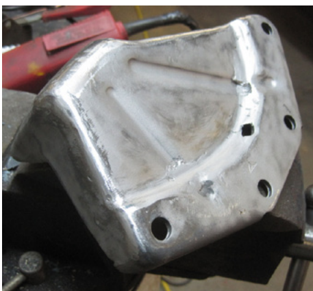
The balancer side of the mount after a 1/4" strip was removed and the remaining parts welded together.
