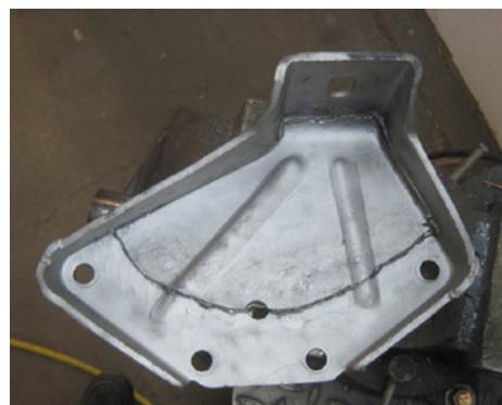
The back side of the mount after all the cutting and welding has been done. The new relief allows space for the fanbelt to fit between the balancer and motor mount.
