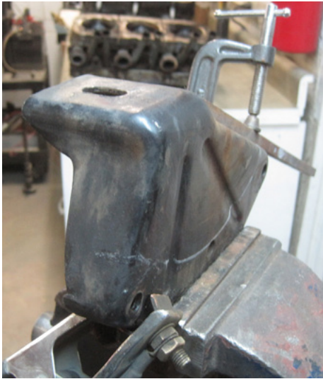
The standard '60-'63 mount is marked for cutting. Use a '64 and later skid plate to mark the curve.
