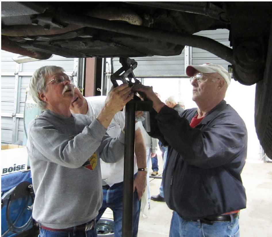
Gary Baxter (left) helps Curt Bonser lower the engine on Curt's '69. The '69 coupe is getting Air Conditioning and they needed to drop the back of the engine to add a pulley to the harmonic balancer to drive the compressor.
