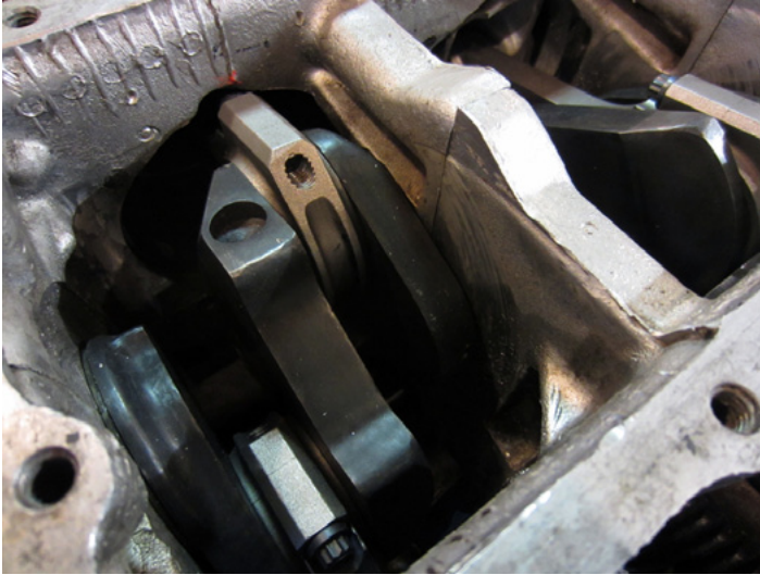
Kevin Willison showed his 3.6 litre Corvair rotating assembly. Special clearancing was required by 1/2" stroke.
