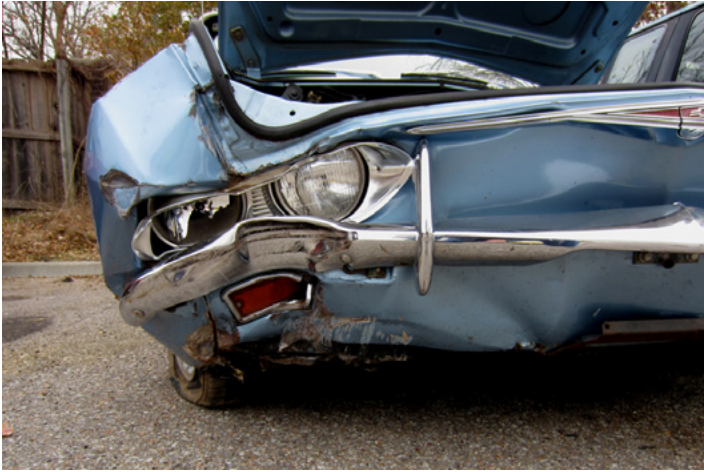
The right front corner took the brunt of the impact. The bumper is flattened where it hit a pole, stopping the car.
