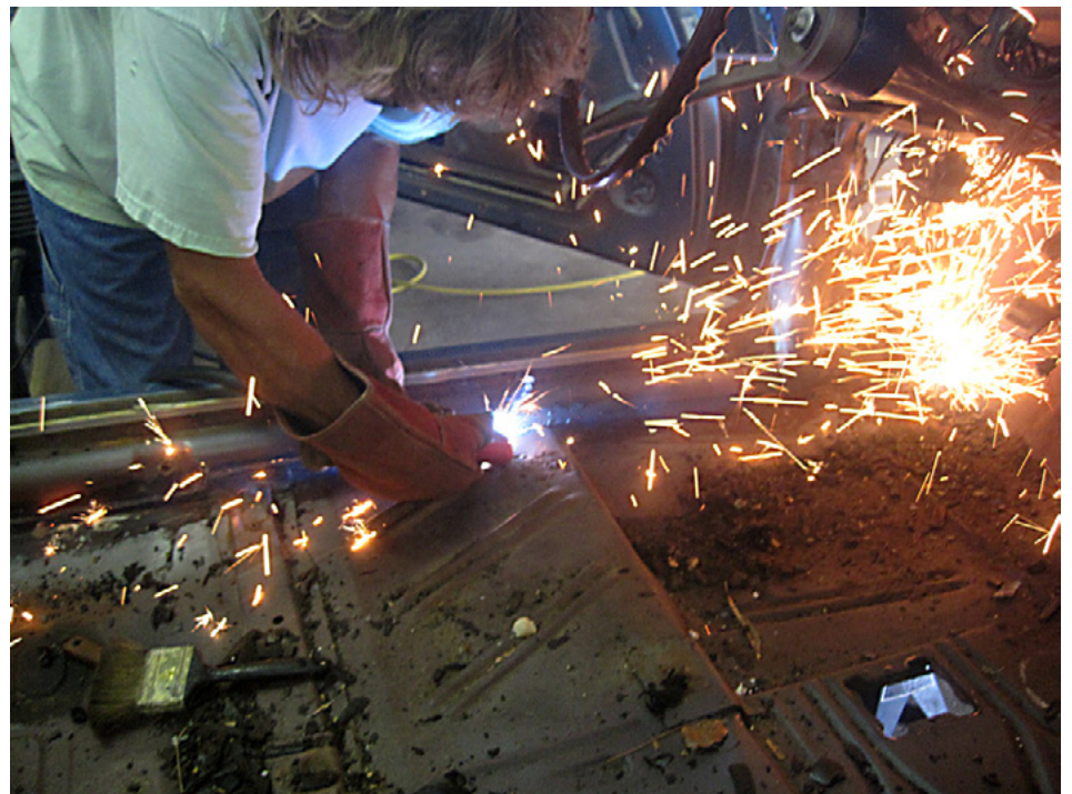
Mike B. of Gypsum, KS (near Salina) is learning to use a plasma cutter at the Kalp Shop. Mike's project was removing the floor from the totaled '65 convertible That Terry is parting out. There are many double and triple layered areas that must be cut before the floor will drop.
