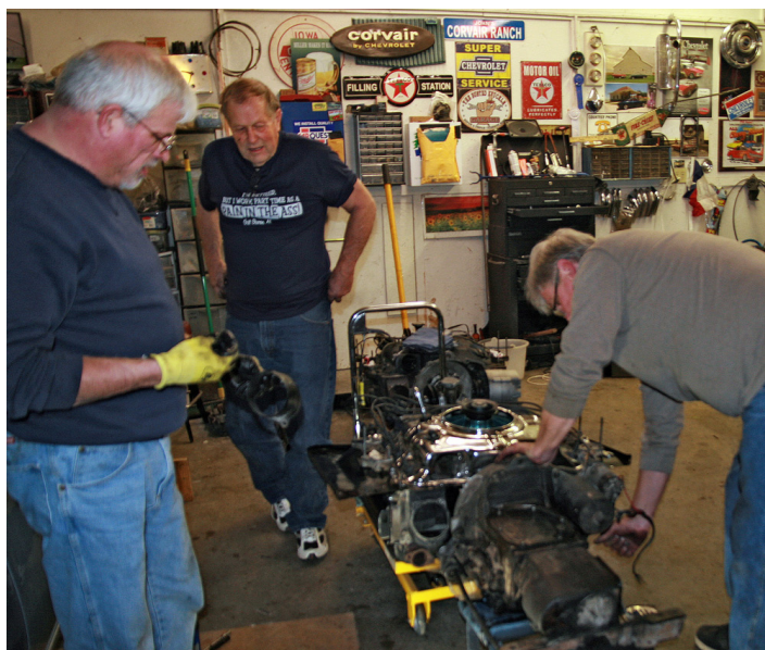
Scott Allison and Gary Jones look on as John Miller prepares the engine to be split from the transaxle.
