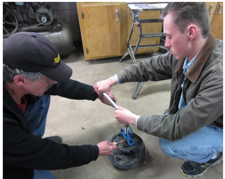
BELOW: DJ and Kota Harms work together to disassemble a LM Corvair rear hub for a disc brake conversion.
