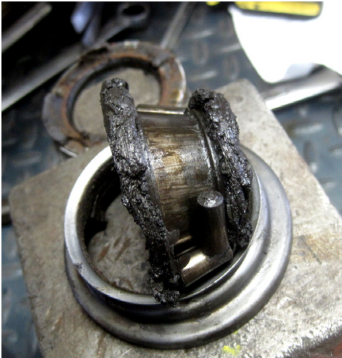
Mark Stever brought his LM rear axle bearings to the Kalp shop for disassembly so the can be cleaned and powder coated. This one wore thru the cage.
