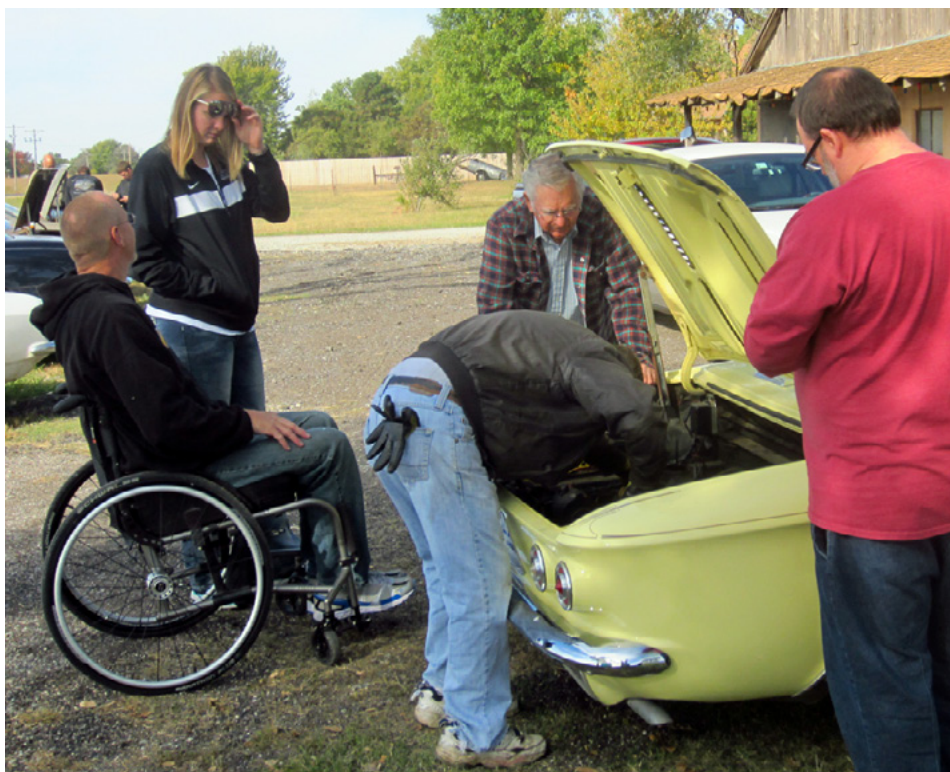
BELOW: Mike Dawson of Kansas City dives into the engine of Lloyd Folger's EM convertible. Mike was working on the carburetor. After some balancing and adjustments, Lloyd's convertible was running much better. Looking on from the left are Mark Stever and his daughter, on the far right is Owen Strawn. .
