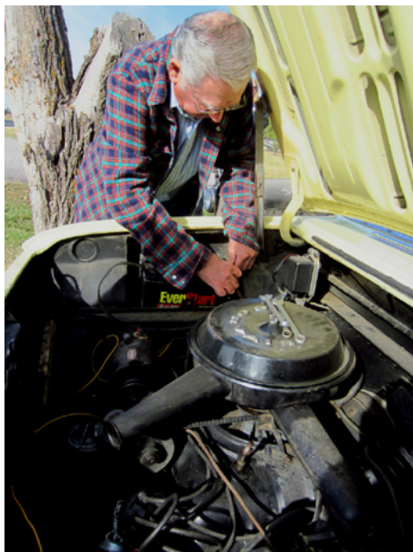
TOP: Loren Capron and James Ergenbright from Oklahoma City, scrub EM rear bearings before repacking them with grease. BOTTOM: Lloyd Folger works on new wiring to give his Pertronix a full 12 volts. Also after a battery cable jumped off on a test drive, he needed to clean and reinstall it.
