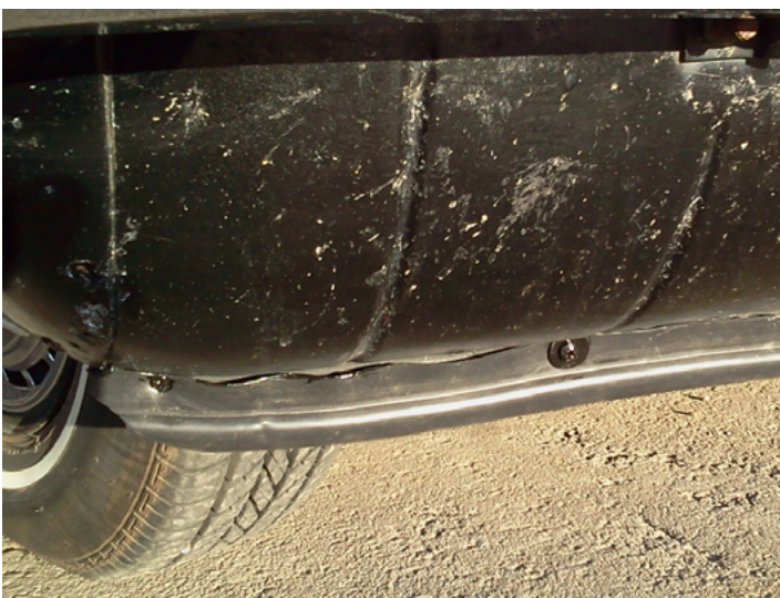
Jens mounted his spoiler with sheet metal screws and a large reinforcing washer to the front pinch weld area of his '64 Spyder coupe.
