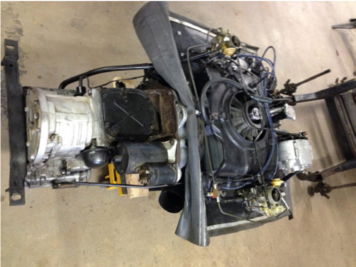
Of course once the engine and transaxle were both together the next logical step was to join them.
