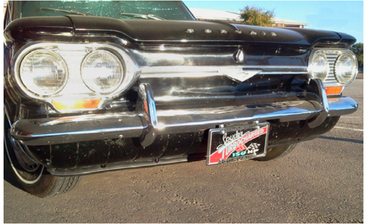
The garden variety spoiler blends in nicely with the Corvair. The depth of the spoiler can be adjusted by how wide you cut it. Jens Mohr photos.
