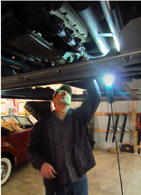
Mark Welte puts the exhaust back together after replacing the manifold to engine donuts that had been leaking.
