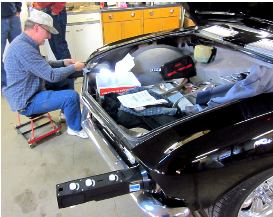
Mark Welte sets up the MCCA headlight aiming equipment. Everything went easier after a broken adjuster was replaced and instructions read.
