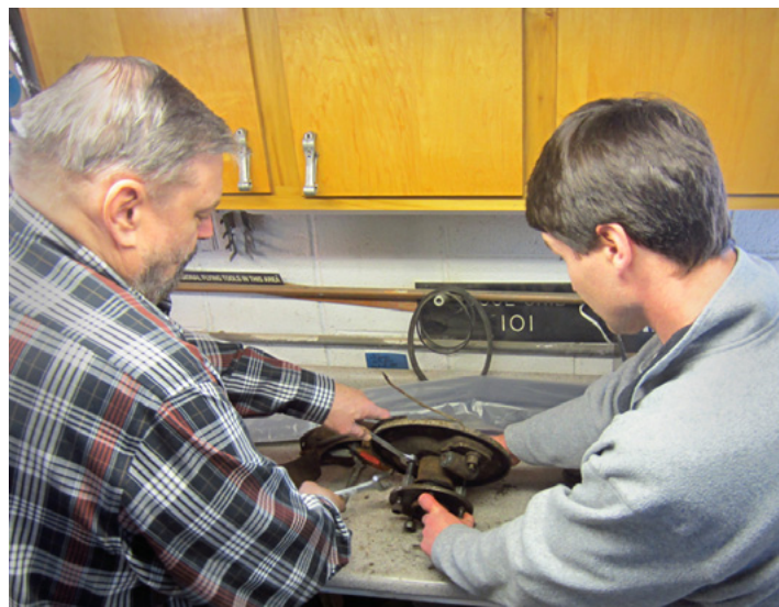
Doug Horstman and Chris Green team up to disassemble a Late Model Corvair rear wheel bearing and hub for Lloyd Folger.
