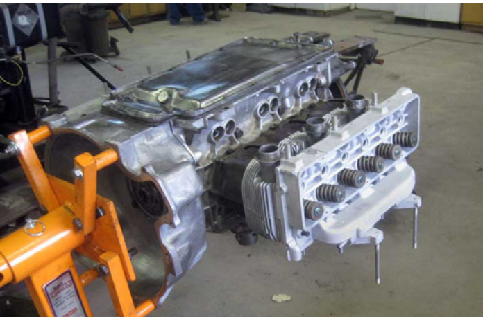
Having the engine upside down made it easier to install the heads. The upper head studs were visible and the push rod tubes were right at hand.
