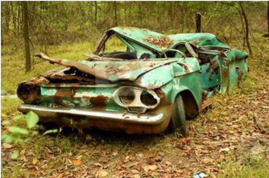
Ran When Parked. Must have been a horrific impact to damage this EM Corvair. Being GM's first unibody car Early Corvairs were overbuilt. Engineers rolled an EM 4 dr several times and the doors still opened.
