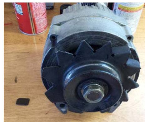
Scotts damaged alternator with one of the "missing" teeth.
