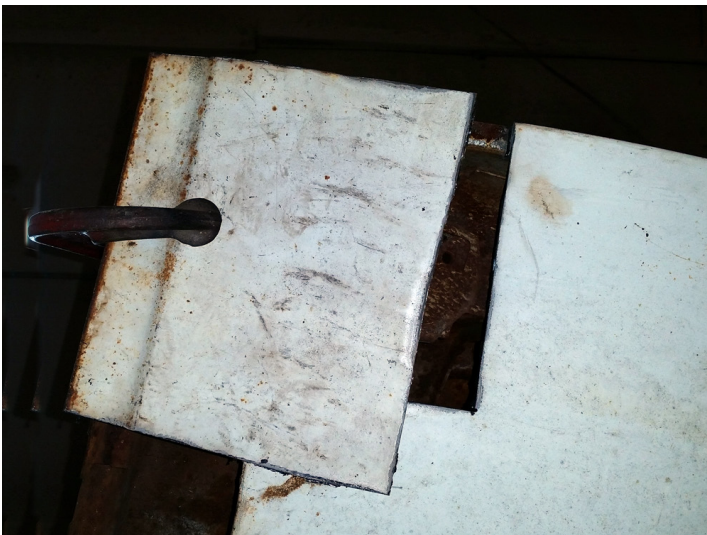
The donor door is put to use again to help form the lip that folds over and crimps the patch panel to the inner frame on two sides. A little heat helps.
