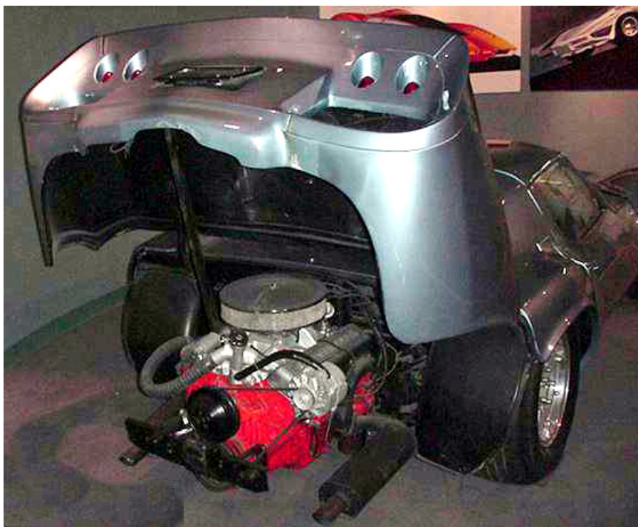
The XP-819, developed in the mid-1960s, was an engineering exercise to test a rear engine concept for the Corvette. The body was designed by Larry Shinoda. You can see styling cues in XP-819 that later appeared in Shinoda's famed "Sting Ray" design. A GM marine engine powers the car so the two-speed transaxle would operate properly.
