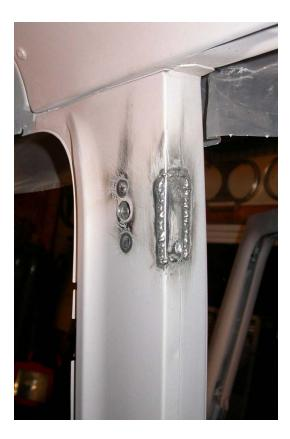
The buckle end belts bolt through a 1/4" reinforcement plate placed in the bulkhead under the seat. The 7" x 2" reinforcement plate is shown here. A small access hole was cut in the front of the bulkhead. Two spot welds had to be removed. To assure proper alignment, 1/8" pilot holes in the plate were used to drill matching pilot holes in the bulkhead; and then expanded to 1/2" diameter. Nuts were welded on back side of the reinforcement plate.
