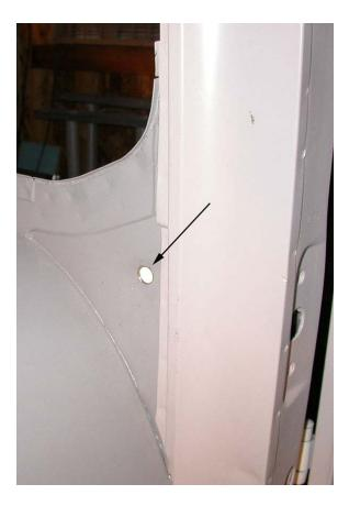
Here is a view from inside the right side wheel well with the retractor bolted through the <sup>1</sup>/<sub>4</sub>" reinforcement plate, which was plug welded in place.
