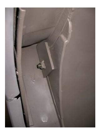
This shows installation of the <sup>1</sup>/4" reinforcement plates for the door post pivots. Using Dremel 409 cutoff wheels, the body skin and interior metal were cut away to allow inserting the reinforcement plate, which has the nut welded on the back side. The bolt hole must be drilled through the interior metal panel to allow the bolt to fully screw in.
