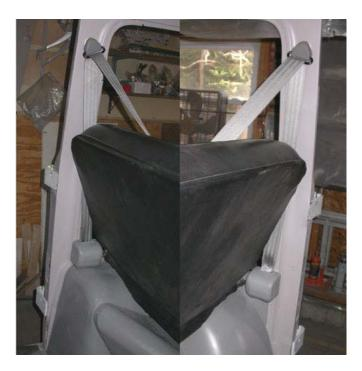
This shows the positions of the buckle ends. The bolt holes are about  $3\frac{1}{2}$  off center.
