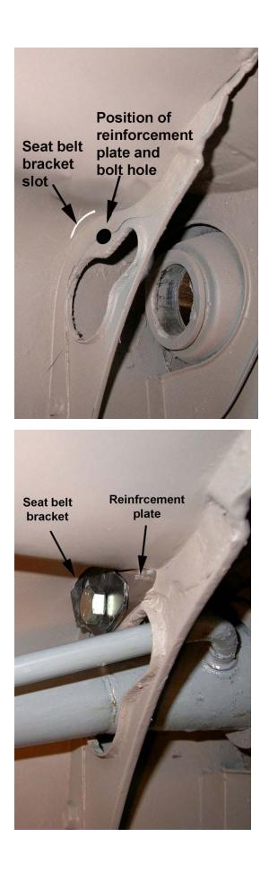
Here is the position of the hole for the right side retractor.
