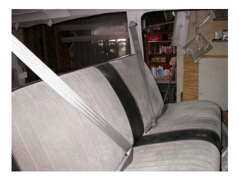
This composite image shows positions of the retractors and door post pivots. The retractors are just behind the furthest rearward position of the seats.
