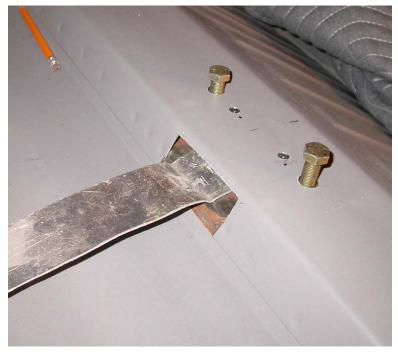
An improvised spatula was used to guide the reinforcement plate into position (very easy), and then the plate was temporarily bolted so that it could be plug welded into place. A replacement plate for the access hole in the bulk head was welded into place and then finished.
