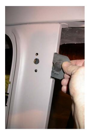
The plate was temporarily bolted and then plug-welded in place. By using the thin cut off wheels, the removed metal can be welded back in place and refinished.
