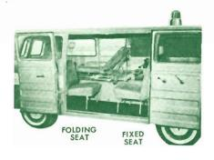
The patient's compartment is 107" long, 41" high, 44" wide - loads of room to accommodate any special equipment such as medicine bar, piped oxygen, auxiliary heater, extra stretcher, etc. The attendant can move about freely to serve his patient - especially good for maternity cases.
