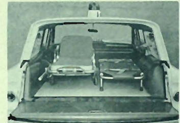
A-602 Cot Holder with special brackets provides width for auxiliary stretcher.
