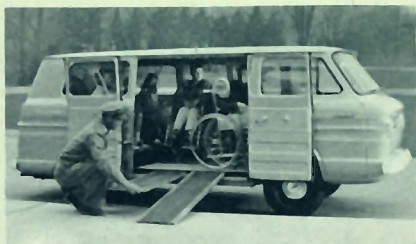
A-661 Self-Storing Entrance Ramp covered with non-skid material and auxiliary floor.
