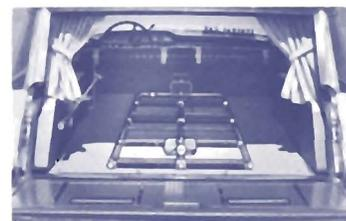
A-601 Casket Rack with adjustable bier pins and A-603 Casket Rollers mounted in tailgate.
