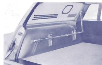
A-6023 Cot Holder with swing back feature which allows second seat to be used without removing cot holder.
