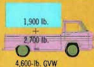
Exceptional payload capacity stems from rugged lightweight construction, with a tough build that carries a full 4,600-lb. GVW rating and a curb weight of only 2,700 to 2,800 lbs. The difference is all payload allowance, 1,900 lbs. in Corvair 95 pickups, 1,800 in the Corvan.
