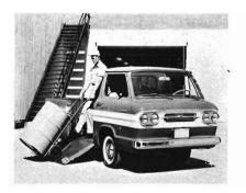
With the Rampside, loading and unloading are even easier. With the ramp gate down, the load can be rolled off or onto the body floor, greatly reducing the need for lifting. The ramp gate is a reinforced, double-panel unit, built to support a 1,600-pound load.
