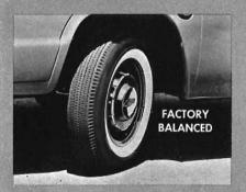
The Corvair 95's 7.00 x 14 tires feature the same improved tread design used on passenger cars. Standard tires carry a four-ply rating. Optional six-ply-rated tires also are available. All tires and wheel assemblies, including the spare, are factory-balanced.
