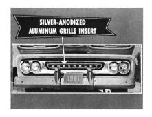
NEW GRILLE DESIGN for 1961 Chevrolet Series 10 through 40 trucks features a stylish, more weather-resistant grille insert in silver-anodized aluminum. The Series 50 through 80 trucks, except tilt cab models, have large, two-digit numbers at the center of the grille, for series identification.
