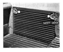
Once closed, the ramp gate can't open accidentally since a safety catch retains the gate positively in the closed position. After the safety catch is disengaged, two release handles permit opening of the gate.
