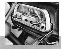
The easy-to-read instruments are recessed under a hood that extends the full length of the panel. When equipped with Powerglide, the shift lever is mounted on the panel alongside a drive-range indicator. Lettering on the speedometer serves as a guide for shifting the optional 4-speed transmission.
