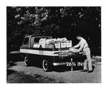
The Loadside Pickup accommodates a big 1,900 pounds of payload in its 80-cubic foot body. With a platform height at the tail gate of only 26½ inches, users will find that loading is extremely easy. The tail gate itself is of sturdy double-wall construction supported with heavy-gauge strap hinges and folding links. The gate is released with recessed corner handles. The double-seal design of the pillars assures a graintight fit.
