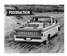
Available as optional equipment for C10 models is the Chevrolet Positraction axle. It provides dependable pulling power even over muddy, icy or rough roads. Positraction keeps these vehicles moving under many conditions which stop trucks with conventional differentials. At the same time it reduces tire wear and drive-line shock loading.
