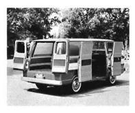
The Corvan has a payload rating of up to 1,800 pounds, a bulk capacity of 191 cubic feet, and a load length of over 10 feet.
