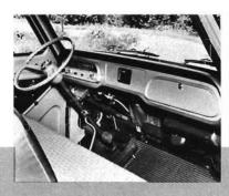
The driver's compartment is both decorative and functional. There is a deep-dish steering wheel and a full-width instrument panel. A dispatch box on the right balances the instrument cluster on the left.
