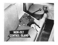
The stationary Non-Tilt Control Island provides shorter, more direct linkage between transmission and gearshift lever, which not only means more positive shifting, but also reduced service maintenance and adjustment.
