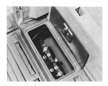
For application in commercial vehicles, 80 gross horsepower and 128 foot-pounds gross torque are completely adequate for meeting tight schedule demands. The twin, single-throat carburetors provide economical power on demand.
