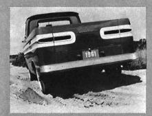
The independent rear suspension features a swing axle with ideal tire-to-road-surface contact. Swing-axle action on uneven surfaces means less "axle hop," reduced power train fatigue, less chassis twist and more positive traction.
