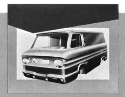
There's integral body and frame construction—body structure and frame formed into one solid integrated unit.
