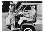
Cab doors open to a wide 85 degrees for easy driver and passenger entry. The driver enters or leaves with a natural sliding action. Once closed, these doors are tightly sealed with closed-cell foam-rubber weather stripping.
