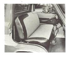
In De Luxe models, seat coverings are checked pattern cloth. Durable nylon with two-tone patterning is used on Custom models. Seat facings are tough vinyl, and the custom seat features a vinyl bolster. A further refinement in the custom seat is extra-thick Polyfoam padding in the cushion and added Polyfoam padding in the back rest.
