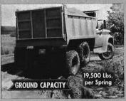
Optional rear spring units on 1961 tandems have been increased to 19,500 pounds ground capacity each, with heavier-gauge spring leaves.
