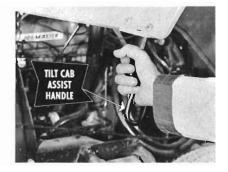
The '61 Chevy Tilt Cab assist handle, conveniently located on the right fender, makes tilting the cab up or down a simple operation.
